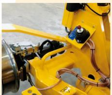
Equipotential bonding according to **RIS1530**
