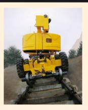
Automatic levelling can operate on 200mm cants with automatic levelling of the turret maintaining a level working position.
