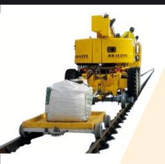
**Towing** hitch and lights pre-arrangement for small trailers.
