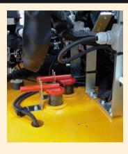
**180 deg turret rotation** restriction by means of mechanical locking pins.
